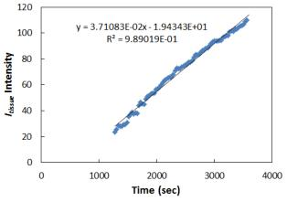
10. The slope of  $I_{tissue}$  is equal to  $I_t/dt$  in Equation [1] to calculate permeability in cm/s. From the example above,  $It/dt = 3.7 \times 10^{-2} \, \text{s}^{-1}$ . For the given example, Equation 1 is calculated:
