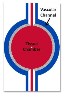
Schematic of the SynTox Model Chip. Vascular channels are for culture of endothelial cells) while thecentral chamber is for culture of tissue cells (smooth muscle cells, fibroblast, hepatocytes, cardiomyocytes, etc.). Porous architecture enables communication between the vascular and tissue cells.
