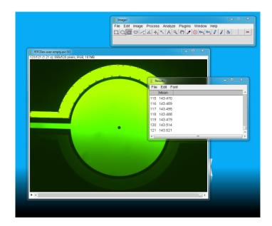
5. Deselect the vascular chamber, and select the tissue chamber using the elliptical selections tool.
