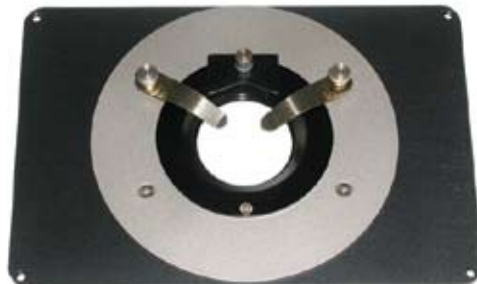
ZEISS TYPE K (160x110mm) leveling x4 set screws in corners
