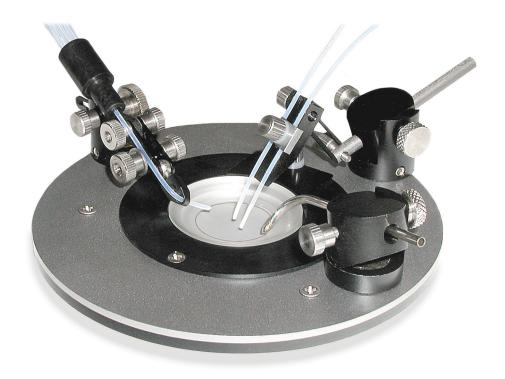
The perfusion manifolds are used to switch between multiple solutions during bath perfusion. This item is included with computerized perfusion systems. The manifold comes with short pieces of PTFE tubing, which fits to polyethylene tubing included with perfusion systems. These pieces can be easily replaced with different tubing of your choice. Use ferrule and luer-type fitting from PS-KIT to attach the manifold to different tubing, including 1/16" and larger I.D. soft tubing.
