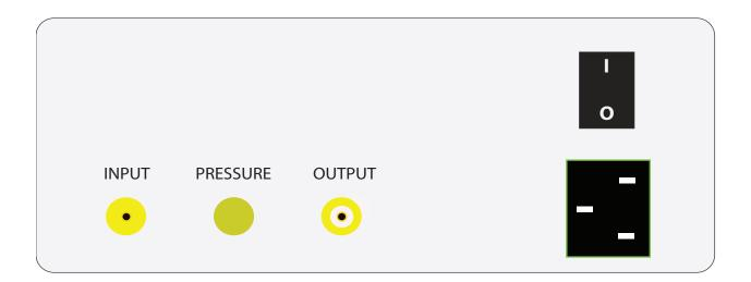
Z Turn the controller ON. The display will show INPUT CLOSED. Rotate the front knob clock-wise to open INPUT port. Although the controller ships adjusted for use with your incubator, it can be re-adjusted using the procedure below.
