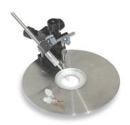
2. The manifold's metal body, a 4 mm O.D. stainless steel, can be mounted on miniature manipulators. The 4 mm rod can be also used to attach the manifold to magnetic holder MTH for small chamber perfusion. The included 7 mm adapter allows you to attach the manifold to regular size manipulators as well.
