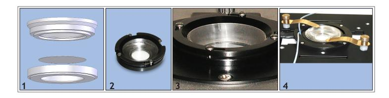
Arrange magnetic holders with inflow manifold and suction tubing around the chamber. While using the cover slips with cultured cells, excess of solution on the cover slip might result in bad seal and cause leakage. Try to leave only a minimum amount of liquid on the cover slip before assembling the chamber.
