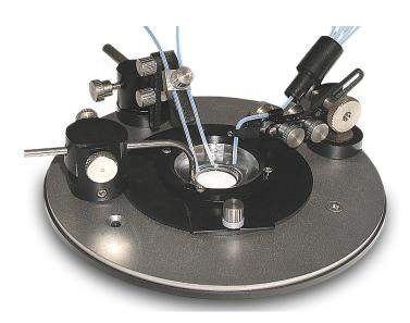
Example of using CSC chamber in a perfusion setup. Magnetic holders are arranged on a microscope adapter MA to provide solution inflow and outflow.
