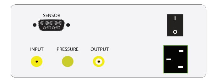
Z Turn the controller ON. The controller will self-calibrate itself for 5min, so make sure there are no residual CO2 under the lid of the incubator. Simply open the lid and let it ventilate for at least 30min. After 5min, The display will show INPUT CLOSED. Rotate the front knob to open INPUT - the controller is ready to use out of the box. Although the controller ships adjusted for use with your incubator, it can be re-adjusted using the procedure below.
