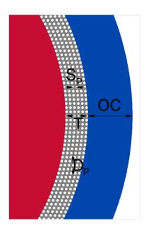
Schematic of the SynRAM model Chip. Vascular channels are for culture of endothelial cells) while the central chamber is for culture of tissue cells (smooth muscle cells, fibroblast, hepatocytes, cardiomyocytes, etc.). Porous architecture enables communication between the vascular and tissue cells and migration of immune cells.
