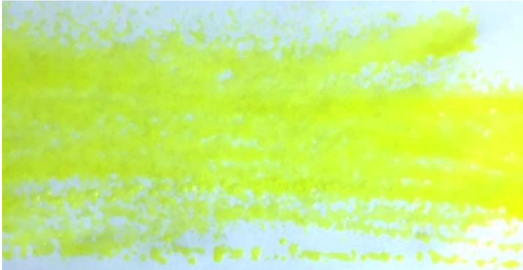
Figure 3-6: A sprayed thin layer of hydrogel using the double barrel syringe and atomizing spray device
